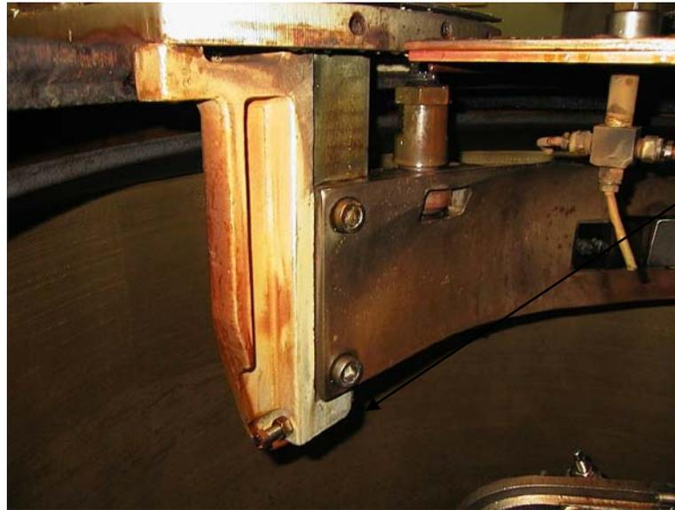
4. Check the condition and finish of the discharger ram. The ram should have a smooth chromed finish free of nicks, burs, and corrosion.
