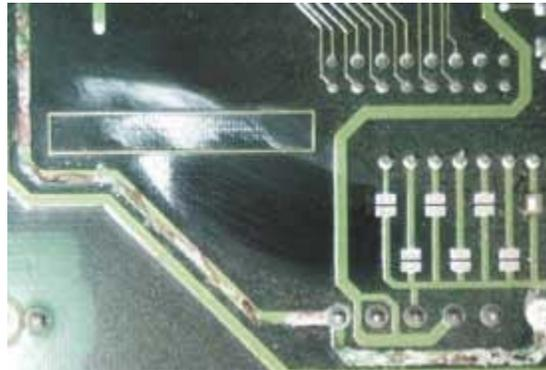
*Fig. 3: Moisture caused corrosion*
